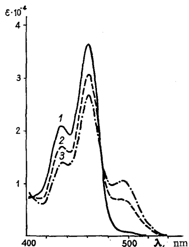
Fig. 1. Absorption spectra of 2-(4-dimethylaminobenzylideno)-5-methylbenzo[b]selenophen-3-one in n-hexane: 1) solution prepared in the dark; 2) solution 1 after irradiation with daylight for 5 min; 3) solution 2 after 10-min irradiation.
